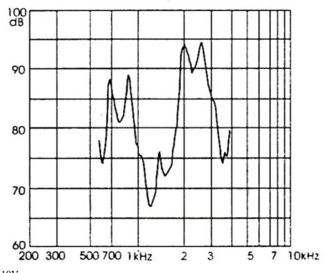
**Note:** Input Voltage 10Vp-p square wave Distance 10 cm
