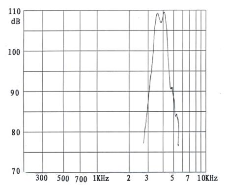
**Note:** Input Voltage 12Vp-p square wave Distance 10 cm
