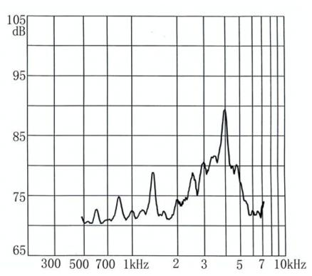
**Note:** Input Voltage 3Vp-p square wave Distance 10 cm
