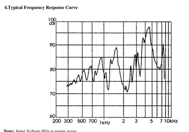
**Note:** Input Voltage 9Vp-p square wave Distance 10 cm
