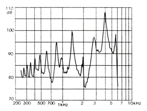
**Note:** Input Voltage 10Vp-p square wave Distance 10 cm
