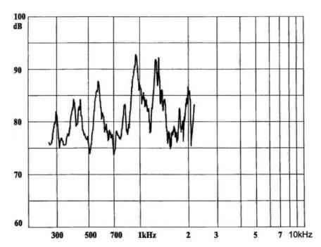
**Note:** Input Voltage 9Vp-p square wave Distance 10 cm
