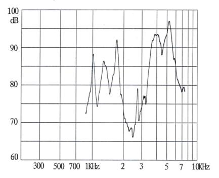
**Note:** Input Voltage 9Vp-p square wave Distance 10 cm
