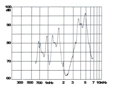
**Note:** Input Voltage 5Vp-p square wave Distance 10 cm
